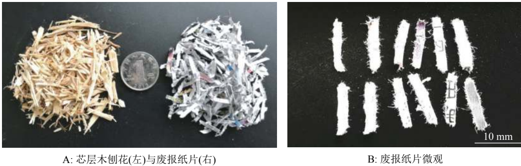
图 1 废报纸片和木刨花形态 Fig. 1 Morphological features of waste newspaper pieces and wood particles
