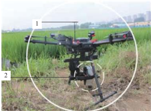
1: M600 PRO 六旋翼无人机; 2: GaiaSky-mini 高光谱成像系统 1: M600 PRO six-rotor UAV; 2: GaiaSky-mini hyperspectral imaging system
