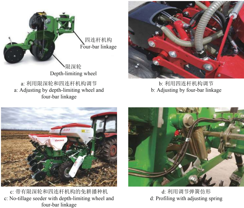
图 9 采用限深轮和四连杆机构控制开沟深度 Fig. 9 Control of rowing depth with depth-limiting wheel and four-bar linkage
