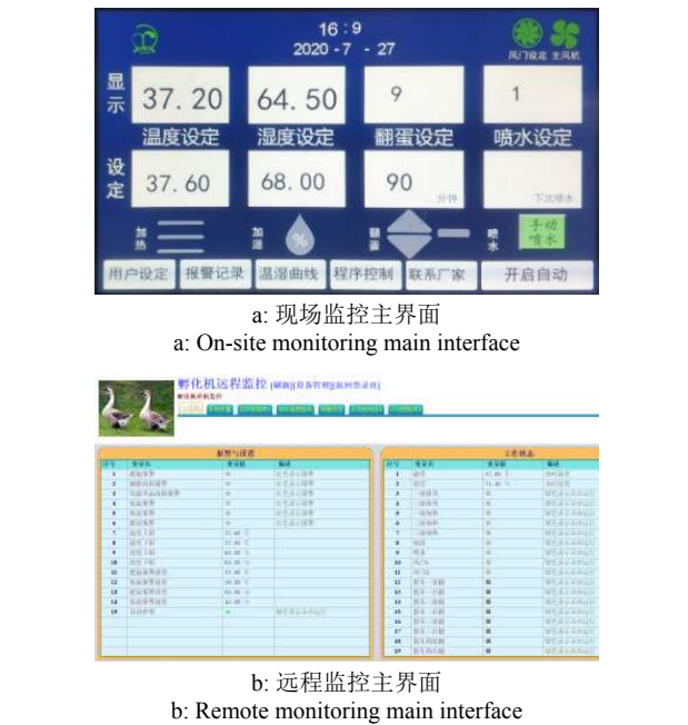
图 9 鹅孵化机监控系统操作界面 Fig. 9 Monitoring system operation interface of the goose incubator
