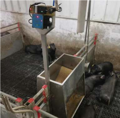
图 7 保育猪/育肥猪小群体粥料饲喂机 Fig. 7 Feeding machine for small group of piglets/ growing-finishing pigs
