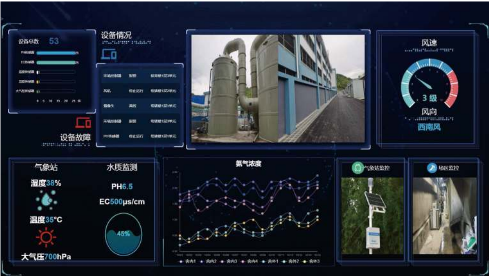
图 3 猪舍环境空气质量智能化管控平台 Fig. 3 Intelligent management and control platform for pig house ambient air quality
