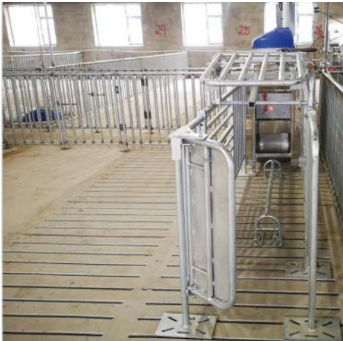
图 6 妊娠母猪小群体精准饲喂站 Fig. 6 Precision feeding station for small group of pregnant sows
