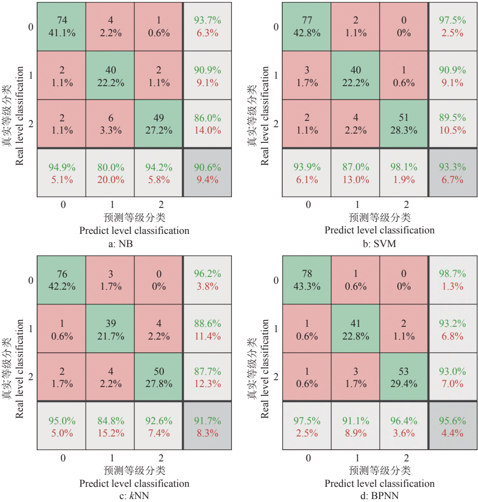
绿色方格代表分类正确样本，其中数字为样本数量和所占总体样本的比例；红色方格代表分类错误样本；浅灰色方格中数字代表测试集样本每一行和列的真相性率（绿色）和假阴性率（红色）；深灰色方格中数字代表测试集样本的总体准确率（绿色）和总体错误率（红色） Green squares represent correctly classified samples, where the numbers are the number of samples and the proportion of the total sample; Red squares represent misclassified samples; The numbers in the light gray squares represent the true positive rate (green) and false negative rate (red) for each row and column of the test set sample; The numbers in the dark gray squares represent the overall accuracy (green) and overall error (red) of the test set samples
