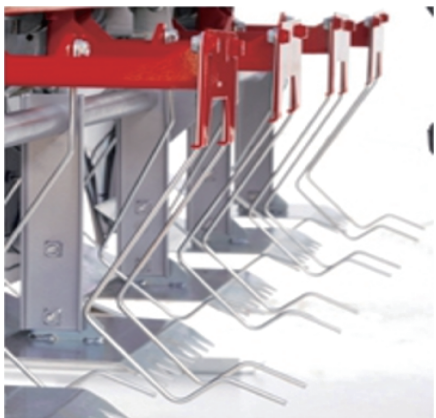
b: 摆动梳齿式株间除草部件 b: Swinging elastic tooth intra-row weeding unit
