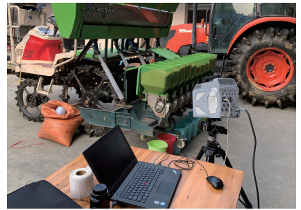
图 5 护种带打滑率试验 Fig. 5 Slip rate test of guard belt
