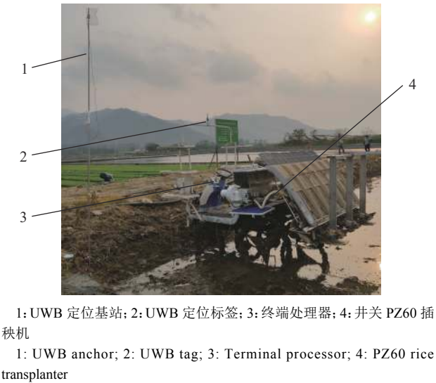
图 8 插秧机搭载辅助导航系统 Fig. 8 Transplanter equipped with auxiliary navigation system
