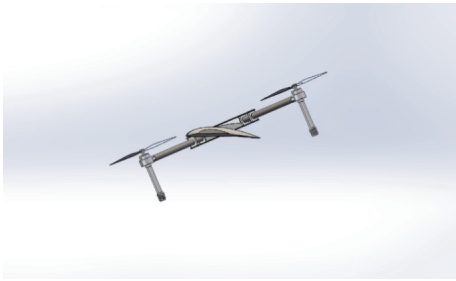
图 2 植保无人机倾转机翼示意图 Fig.2 The diagram of tilting wing of plant protection UAV
