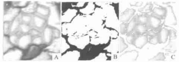
A: 灰度图像; B: 阈值分割的二值化图像; C: 图像分割结果 A: gray image; B: black and white image by threshold segmentation; C: result of image segmentation
